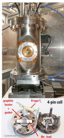
4-pin resistive heating cells and vacuum chamber
