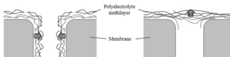
Polyelectrolyte layer-by-layer coating of membrane pores for drinking water treatment
