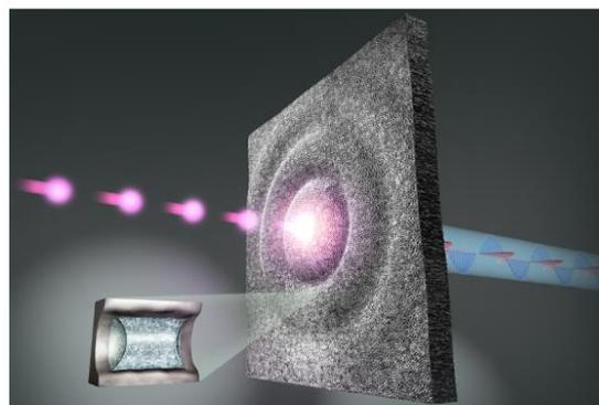
Laser-ultrasound experiment on water-infiltrated nanoporous silicon. (TUHH/DESY/Künsting)
